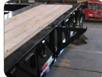
Standard heavy duty outriggers that span the entire height of the side rail allow for maximum force to be applied when in use.
